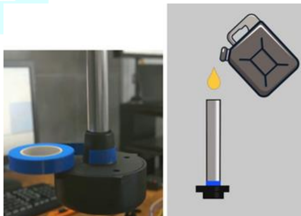
Closing drain holes, rotating sensor, and filling tube with fuel
