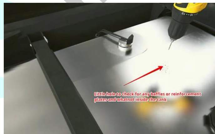
Drilling the tank and subsequent examination of the tank for the presence of obstructions
